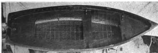
A 14-foot rowing boat arranged to be used as a yacht tender. Bronze trimmings
